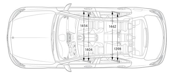
All figures in millimetres. The illustrated dimensions are mean values, They are valid for vehicles in basic specification and in unladen condition.
